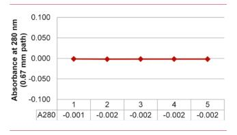
Figure 4: No carryover is detected. Absorbance at 280 nm (0.67 mm path) of five 1x PBS measurements measured after the last protein sample.
