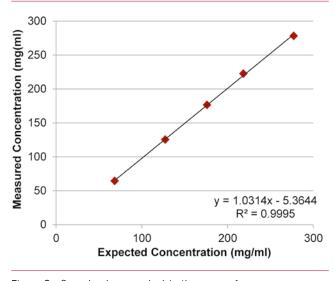
Figure 3: Samples (mean value) in the range of 68.326 – 276.98 mg/ml were measured with path length 0.07 mm.
