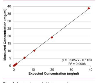
Figure 2: Samples (mean value) in the range of 0.038 – 39.097 mg/ml were measured with path length 0.67 mm.
